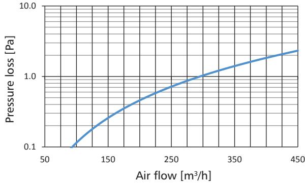
Measurement: inner diameter: 180mm, length: 1m,
