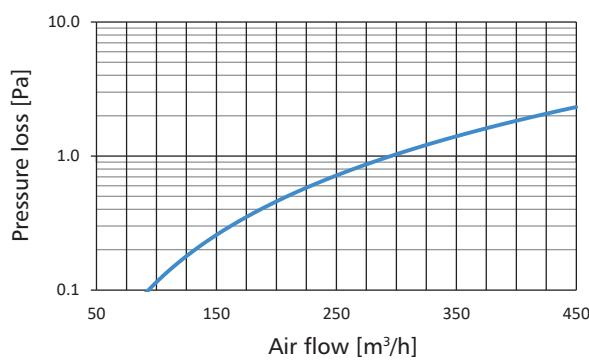
Measurement: inner diameter: 160mm, length: 0.5m, temp: 30.6°C,  $P_{atm}$ : 1004 mBar,  $\rho$  (density): 1.151 kg/m<sup>3</sup>
