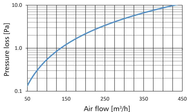
Measurement: inner diameter: 150mm, length: 1m, temp: 28.5°C,  $P_{atm}$ : 1004 mBar,  $\rho$  (density): 1.159 kg/m<sup>3</sup>
