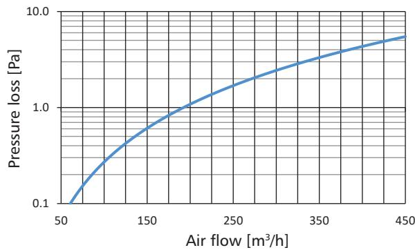
Measurement: inner diameter: 150mm, length: 0.5m, temp: 28.5°C,  $P_{atm}$ : 1004 mBar,  $\rho$  (density): 1.159 kg/m<sup>3</sup>
