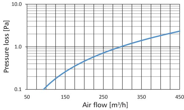
Measurement: inner diameter: 125mm, length: 1m, temp: 25°C,  $P_{atm}$ : 1004 mBar,  $\rho$  (density): 1.173 kg/m<sup>3</sup>
