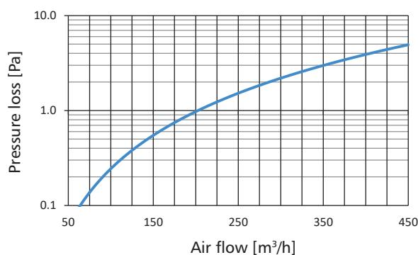
Measurement: inner diameter: 160mm, length: 1m, temp: 30.6°C,  $P_{atm}$ : 1004 mBar,  $\rho$  (density): 1.151 kg/m<sup>3</sup>
